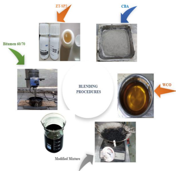
Fig. 2. Blending procedures of modified samples
