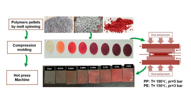
Fig. 1. Schematic diagram for the fabrication of fluorescent polymeric thin films by the hot-pressing mechanism under specific temperature and pressure
