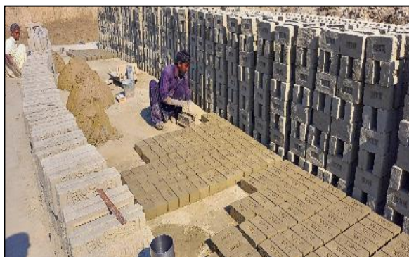
Fig. 5. Molding of Bricks
