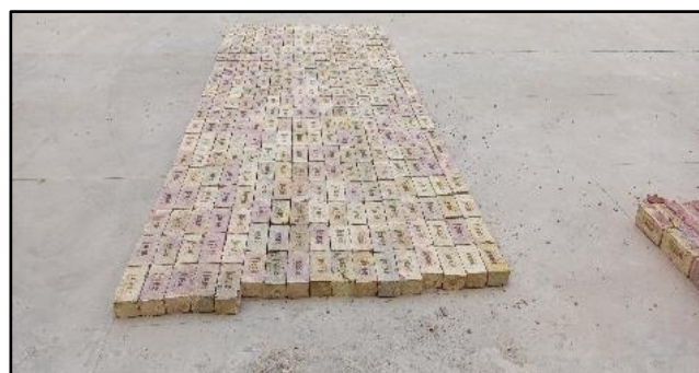
Fig. 24. Dimensional Tolerance Test
