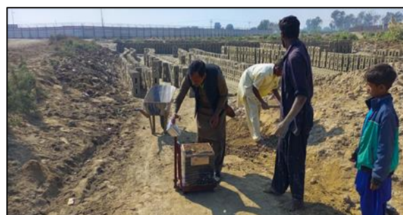
Fig. 3. Determination of Soil Weight
