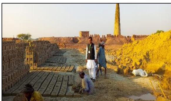
Fig. 6. Setting up Bricks for Drying
