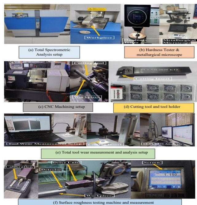
Fig. 1. Overview of the experimental setup and characterization equipment used in the machining setup
