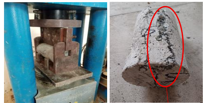
Tensile Failure Pattern
