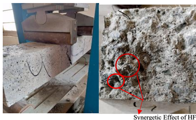
Fig. 8: Overview of Flexural Strength Testing & Results
