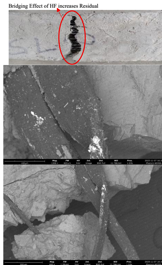
Fig. 9. SEM Images of RNF in Concrete Matrix
