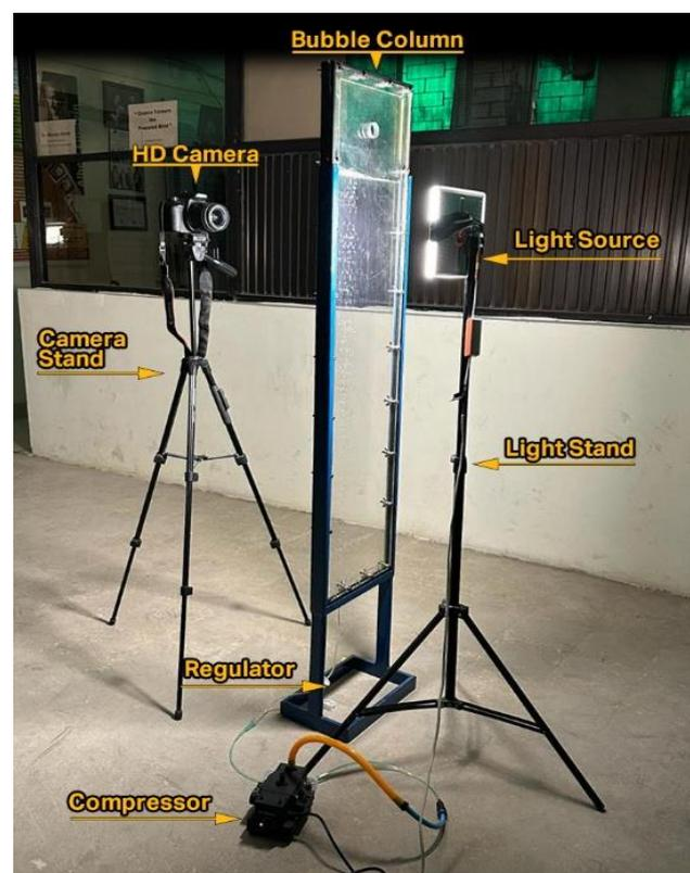
**Fig. 3.** Bubble column Exp Setup
