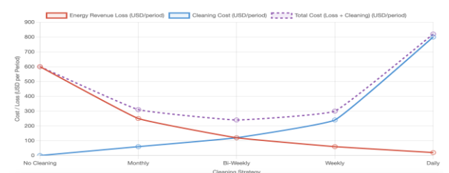
Fig. 7. Cost-Benefit Graph: Cleaning Cost vs Energy Revenue Loss
