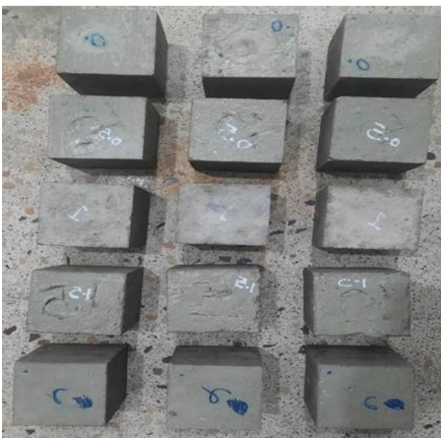
Fig. 6. Physical inspection of self-curing concrete on the 1 st day of concrete age
