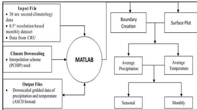
**Fig. 1** Flow Chart Describing Method For Determining Historic Precipitation And Temperature Data (1950 - 2000)
