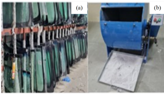
Fig. 2. Preparation of materials (a) Automotive glass waste (b) Grinding machine
