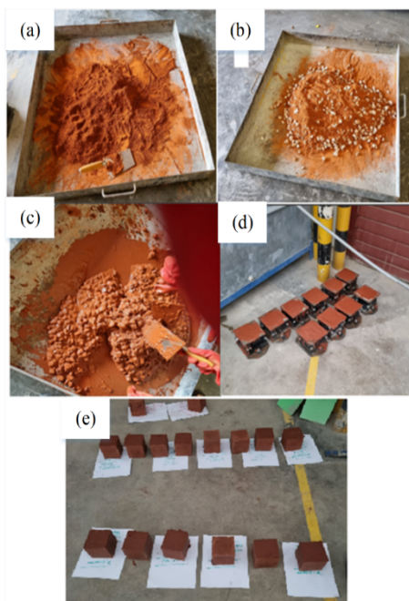
Fig. 6. Casting process (a) Dry mixture of binder materials, (b) Dry mixture of GPC ingredients, (c) Mixing of GPC ingredients with alkaline solution, (d) Fresh GPC cubes in the moulds, (e) Ambient curing of GPC cubes after demoulding
