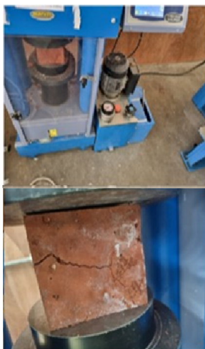
Fig. 7. Compressive strength test of GPC cube
