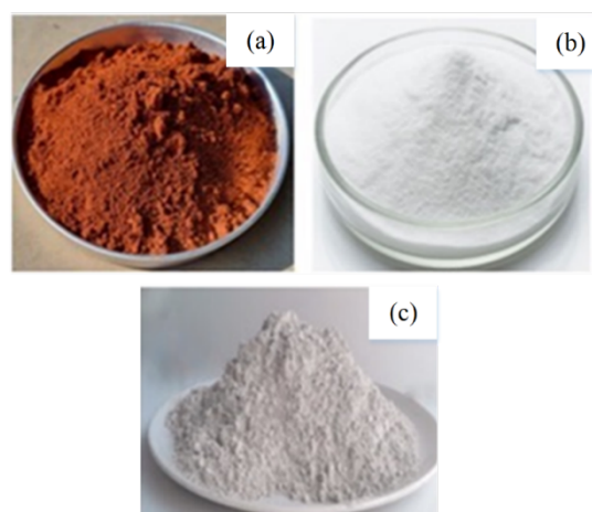
Fig. 1. Binder materials: (a) RM, (b) AGWP, and (c) GGBFS
